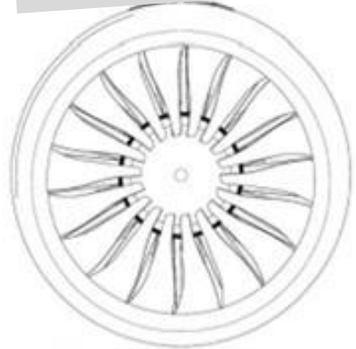
Next A/C generation > 2025 : UHBR Fan diameter : > 80'' Bypass ratio : > 12 smallest nacelle
