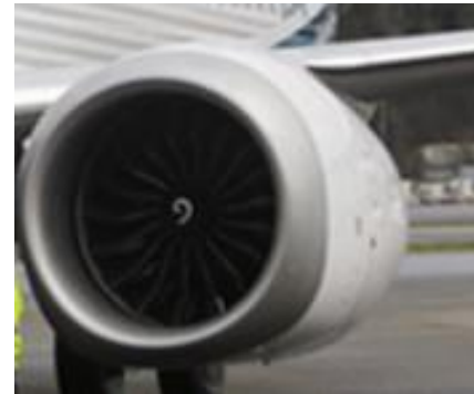
2017 : LEAP-1B Fan diameter : 69'' Bypass ratio : 9
