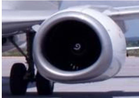
1998 : CFM56-7B Fan diameter : 61'' Bypass ratio : 5,5
